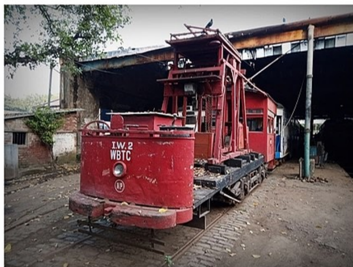
A pre-independence built Overhead Equipment Inspection Tram still in service Photo by Rudranil Roy Chowdhury
