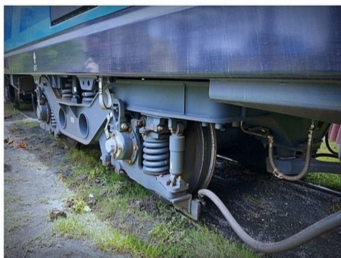
The goose-neck shaped sole-bar...
