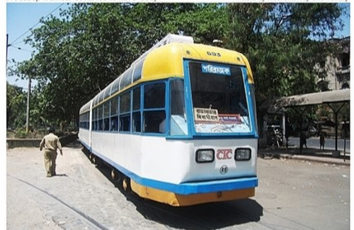
A Jessop tramcar converted to fibre-body
