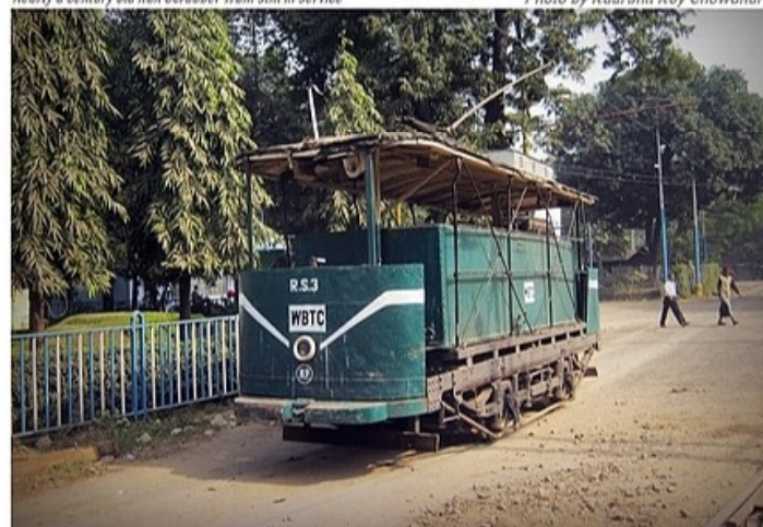
Nearly a century old Rail Scrubber Tram still in service
