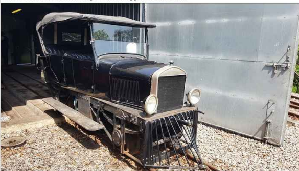
Model T Petrol Car - Undoubtedly the BLR's most unusual item of motive power. Still with its original engine and fitted with a turntable allowing the car to be raised from the rails, turned and then lowered to face in the opposite direction.
