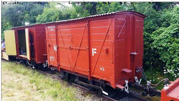
The BLR had a small but interesting fleet of freight stock. These two box vans (fitted with twin-pipe air brakes) were previously in Royal Navy service at an armament depot.
