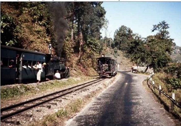
In one of the passing loops allowing a downhill train to pass
