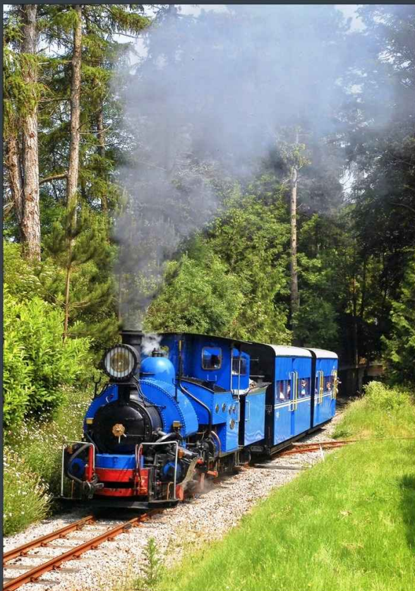
The loco, built by Sharp Stewart, is largely original, still retaining its 1889 boiler. The tender carries the coal (rather than DHR-style above the boiler) and fittings for vacuum and air brakes.
