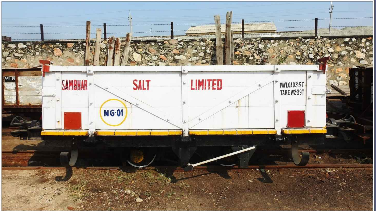
A NG salt wagon numbered NG-01 from Sambhar Salts Ltd. Tare Weight or weight of the wagon in empty state is 2.39 T & Payload or weight of the wagon in loaded state is 3.5 T. These wagons have been manufactured by Braithwaite & Co. limited (Ministry of Railways) & relatively new.
