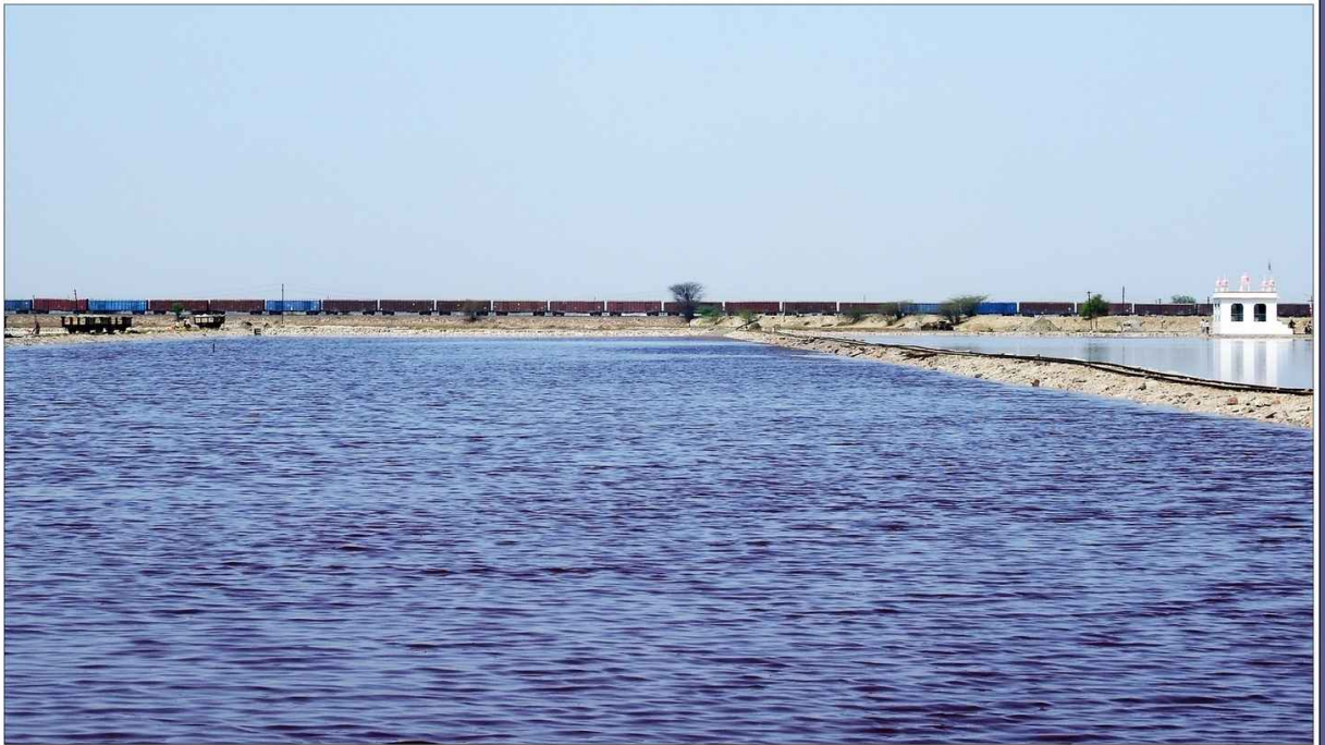
A water filled sat bed & a BCNA rake in the backdrop. The water has a light reddish tinge which is an indication of lesser quantity of algae & henceforth, lesser amount of salt formation.
