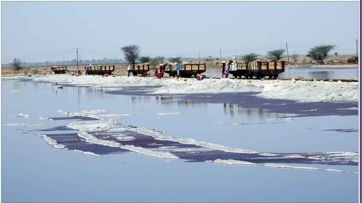
MG wagons scattered parallel to the salt bed. Raw-unfiltered salt is being collected in the wagons at different points to facilitate faster loading.
