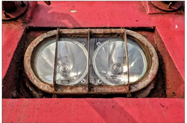
Twin-Filament Twin-Beam Halogen Headlamp Setup on a WAP4 class locomotive
