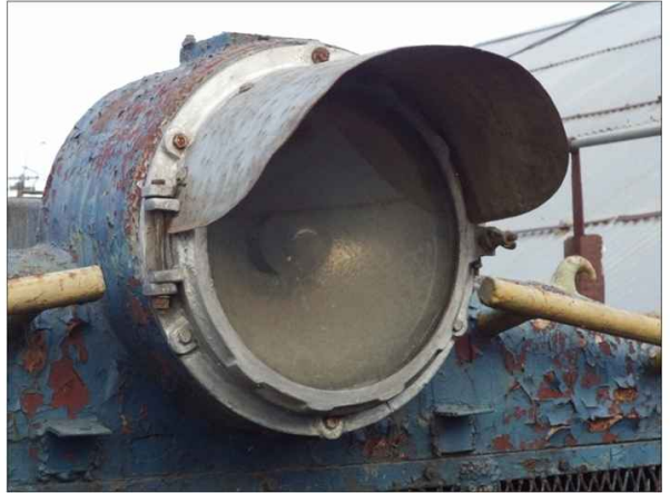
Single beam headlamp fixture on an NG locomotive
