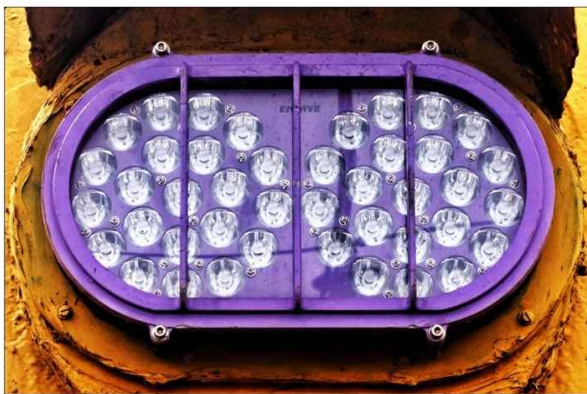
LED Twin Beam Lamp Setup on a Dual Mode Shunter converted from a MEMU by KPAW
