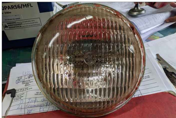
A single unit of PAR56 bulb, especially for G9, P7 & P5 Locomotives
