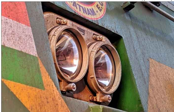
VSKP(D) WAG9HC 33367 with clear lens type PAR56 lamps
