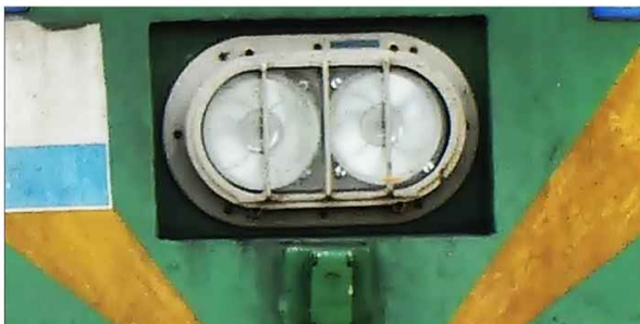
GMO WAG9 31308 with H4 Halogen lamps
