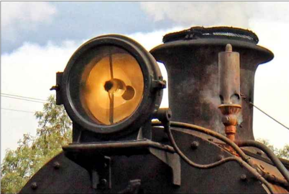
Inverted headlamp fixtures fitted on a steam locomotive
