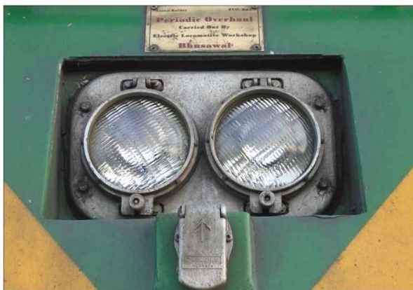
Headlamp of WAG9 locomotive with Twin single filament PAR56 lamps
