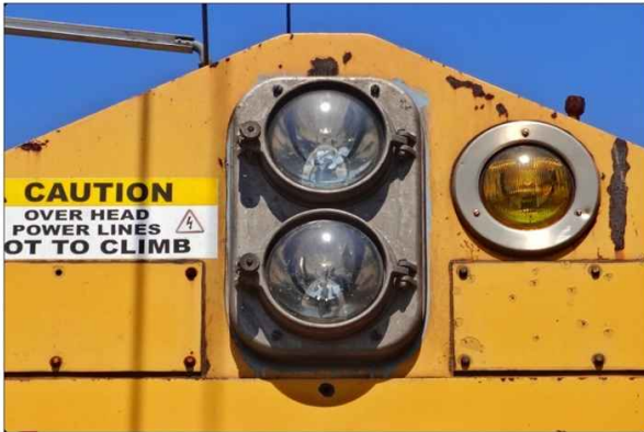
Headlamp of WDG4 Locomotive with Two Single Filament PAR56 Clear Glass Bulb
