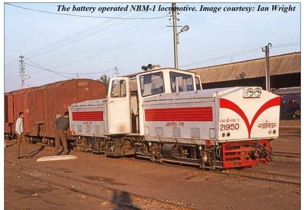
The battery operated NBM-1 locomotive. Image courtesy: Ian Wright
