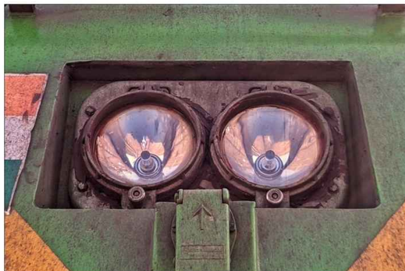
GMO WAG9 31022 "NAVYUG" with the H4 Halogen lamps
