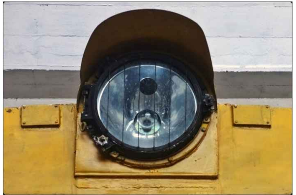
Twin Lamp Single beam headlamp fixture on a Kolkata Metro Railway Inspection Car
