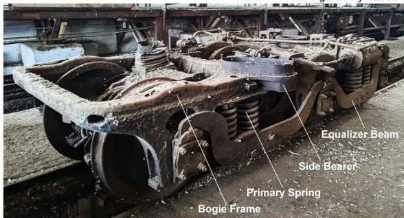
Co-Co wheel arrangement of a YDM-4
