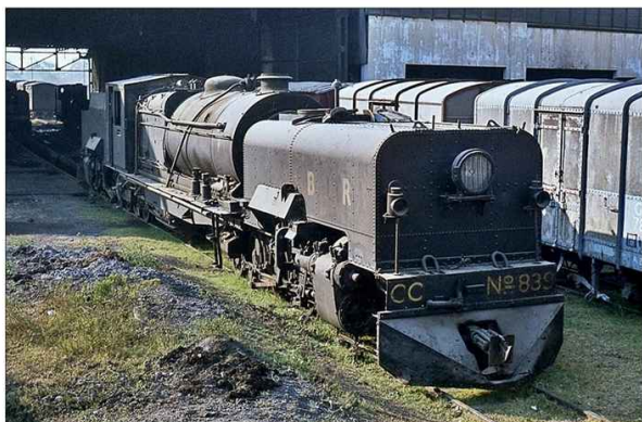
Last 2-8-2+2-8-2 MWGH Garratt in Burma as GC Class No. 839. Photo by Mark Carter
