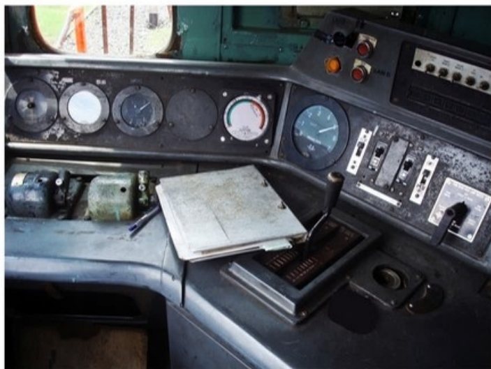
Conventional Driving Panel of a WDM3D Locomotive
