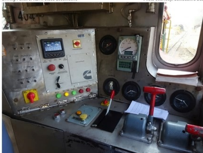
Driving Panel of NDM1 Class Locomotive
