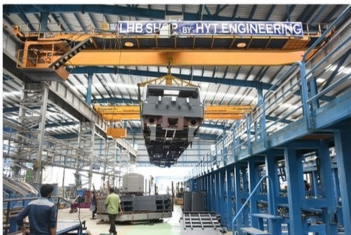
Lifting of the Driving Trailer Car (DTC)
