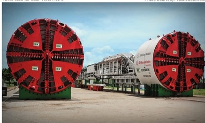
TBMs used for East-West Metro
