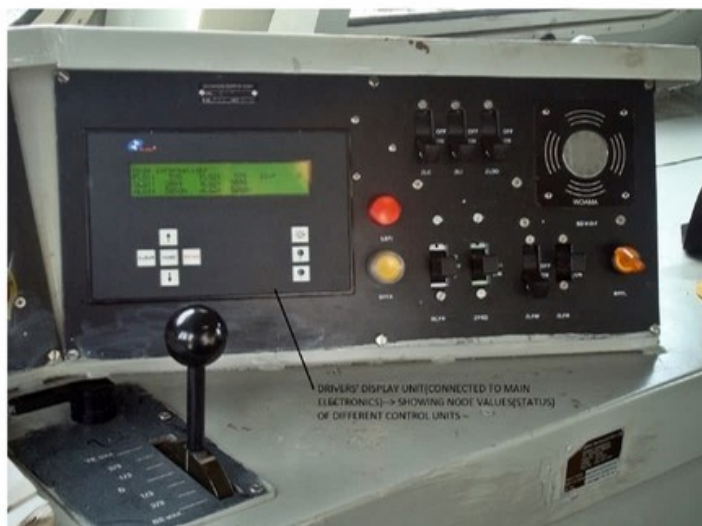
Driver's Display Unit of a 3-phase Locomotive
